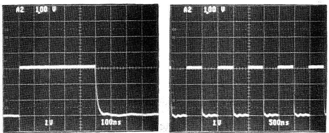
Input Voltage=950V, Pulse Width=100ns, Pulse Recurrence
