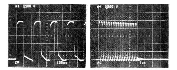
Input Voltage=950V, Pulse Width=200ns, Pulse Recurrence Frequency=500Hz, Oscilloscope Scale=1000V/DIV, Load=1000 ohm in secondary:
