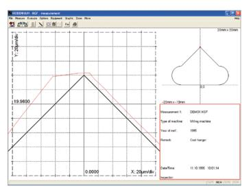
Standardized representation of a free-form test with a KGM and detail zoom: here a normal view shows an overshoot with the resulting rounding-off error (nominal path in black, actual path in red).
