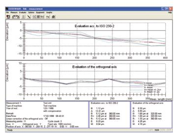
Measurement of the static positioning accuracy as per ISO 230-2 and the guideway error in transverse direction with the VM 182
