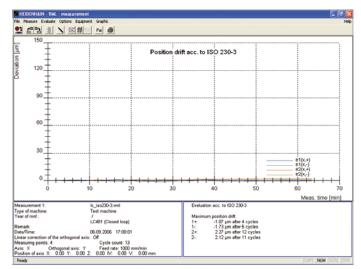
... ... or for feedback from a linear encoder (Closed Loop)
