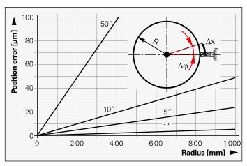
Influence of the distance R of the machining position from the center of the rotary table on the positioning accuracy  $\Delta x$  at various angular errors  $\Delta \phi$  of the rotary table
