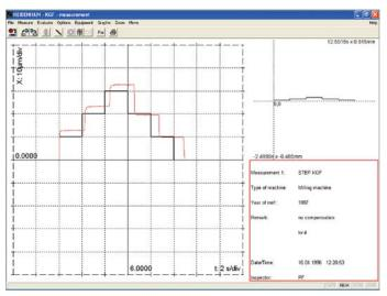
Result of a step response test as an "Xt" graph
