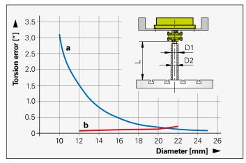
Torsion error of the 100 mm long coupling of an ROD 880 through a a) Solid shaft with various diameters D1
