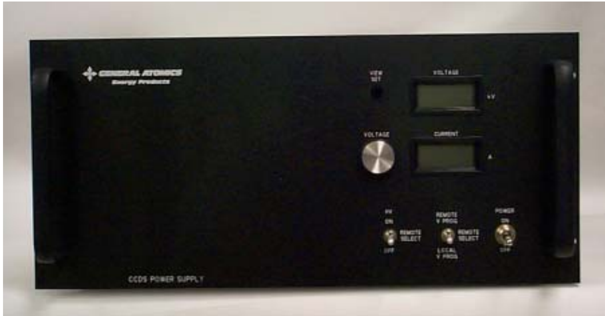
Figure 5-1. CCS High Voltage Power Supply Front Panel – Instrumented.
