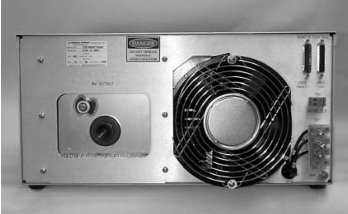
Figure 5-2. Typical CCS High Voltage Power Supply Rear Panel.
