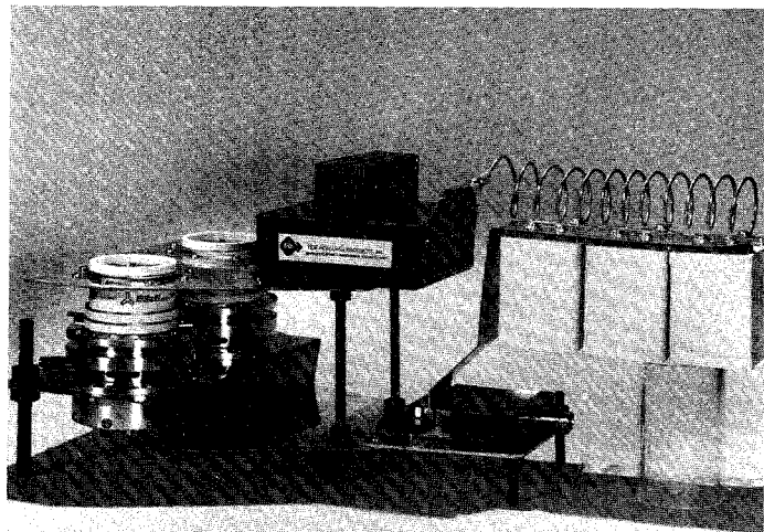
Fig. 2. Parallel tube test circuit.
