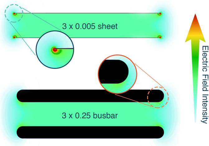
Cutting conductors from sheet metal is a common expedient for making wide planar transmission line conductors, but sheet metal has inherently sharp edges that lead to electric field enhancement and breakdown unless the conductors are widely spaced. Spacing the conductors of a transmission line far apart to prevent dielectric breakdown is at odds with achieving fast rise time for a low impedance load because distance between conductors increases inductance.
