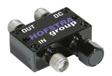
The 4204 Impulse Forming Network (IFN) differentiates fast voltage steps into picosecond impulses in a single compact and reliable module. With an integrated DC bias injection port, the 4204 IFN is perfectly suited for driving and biasing diode lasers.
